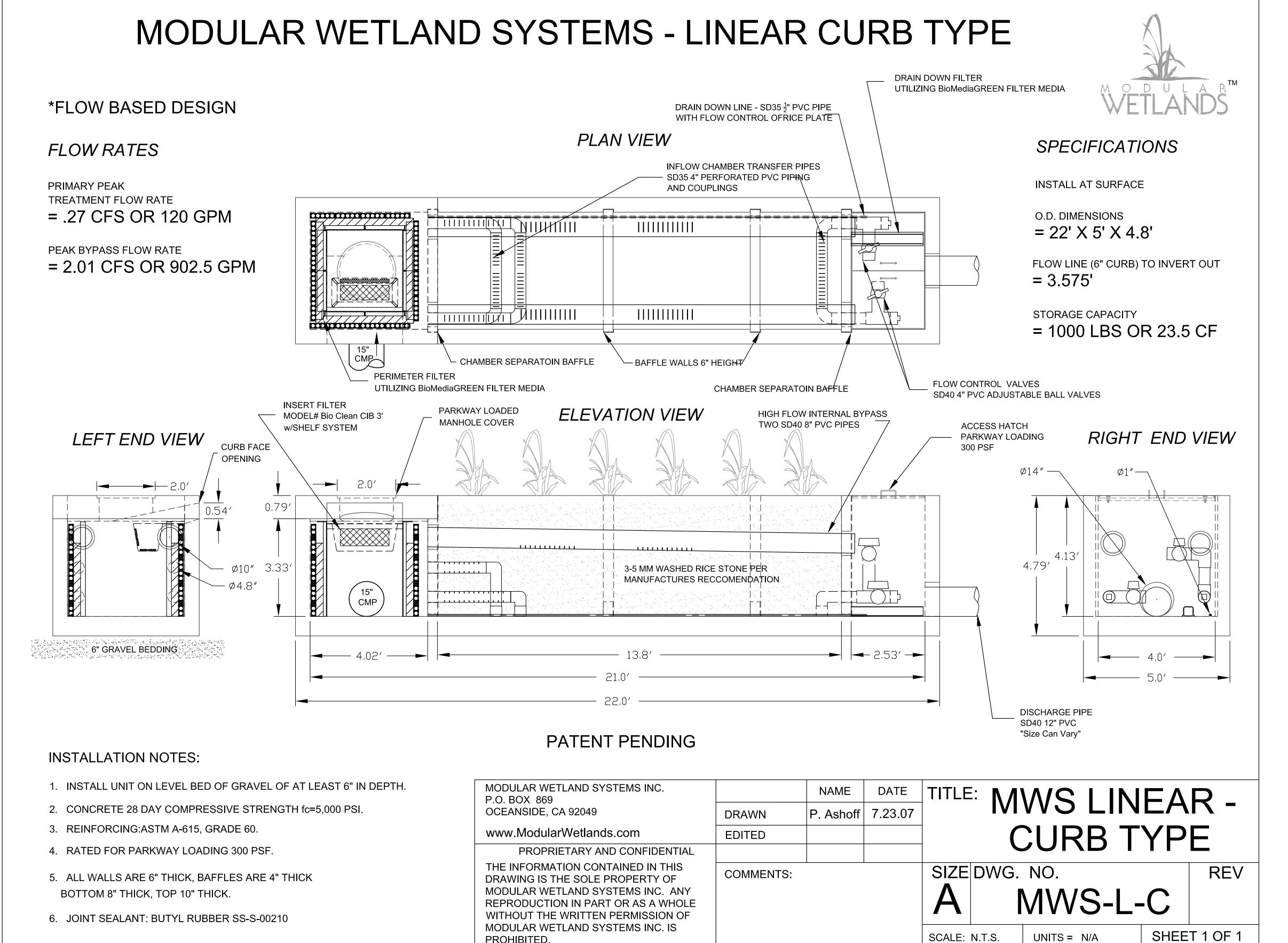
TYPICAL SCHEMATIC MODULAR WETLAND SYSTEMS (LINEAR CURB TYPE)
